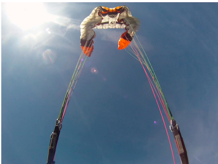
Careful! Swinging backwards means you'll pendulum! If you put your hands up at this stage, the wing will start to fly again, violently. The pendular conversion will be combined with an aerodynamic conversion, the surge will be very strong and you could fall into the wing! Keep your hands locked until the pendulum movement has calmed down.
