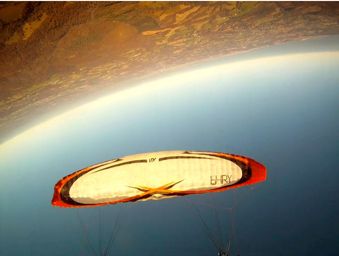
With the wing at 30° in front of you, you can damp it out with a short hard pull on the brakes...
