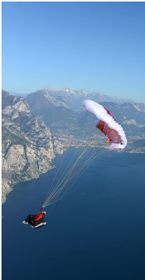
A NICE STALL SEQUENCE. THE PILOT SLOWS, SLOWS...THE WING STOPS FLYING AND STOPS SUPPORTING HIM.
