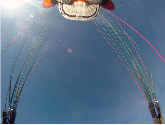
The wing starts its stall. The Dolpo has the peculiarity that it clearly starts to stall from the wing tips.
